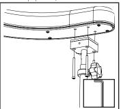
4. Flip the ratchet lever over and place it over the pin and verify the end of the spring is in the hole of the ratchet lever.
