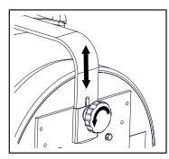
6. To adjust the position of the back, loosen the knob under the seat, slide the back in or out, and tighten the knob.
