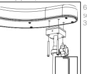
6. Reattach the body support ratchet using the 3/16" Allen wrench
