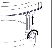
4. To adjust the height of the body support, loosen the knob on the side of the body support, adjust the height, and tighten the knob.
