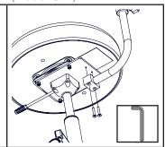
3. Attach the body support tube to the bracket on the underside of the seat with (2) 1-1/2" flat head screws using a 5/32" Allen wrench. Insert the rod of the ratchet assembly into the body support tube with the flat side towards the knob and tighten it into place.
