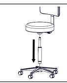
2. Install the larger end of the gas spring into the base of the stool. Place the seat of the stool on top of the gas spring. Sit on the stool to secure the pieces.
