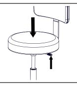
2. To lower the height of the stool, lift up on the lever below the seat while placing weight on the seat.
