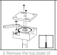
the ratchet assembly, held with two screws, using a phillips screwdriver. Remove the black plastic washer. (It may stick to the bottom of the top plate).
