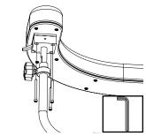
1. Remove the three bolts that secure the body support ratchet to the body support cushion using a 3/16" Allen wrench.
