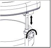
4. To adjust the height of the body support, loosen the knob(s) on the side of the body support, adjust the height, and tighten the knob.
