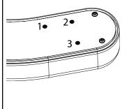
2. Feel for 3 holes hidden under upholstery on the opposite side of the body support cushion. Pierce 3 holes through the upholstery using a sharp instrument.
