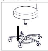
1. To raise the height of the stool, press down or lift up on the foot ring with no weight on the seat.
