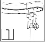
6. Reattach the body support ratchet using the 3/16" Allen wrench.
