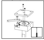
3. Remove the top plate of the ratchet assembly, held with two screws, using a phillips screwdriver. Remove the black plastic washer. (It may stick to the bottom of the top plate).
