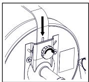
1. Insert the backrest into the bracket on the underside of the seat. Tighten in place with the knob.
