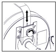
5. To adjust the position of the back, loosen the knob under the seat, slide the back in or out, and tighten the knob.
