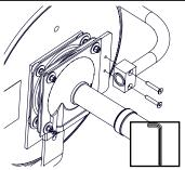
2. Attach the body support tube to the bracket on the underside of the seat with (2) 1-1/2" flat head screws using a 5/32" Allen wrench. Insert the rod of the ratchet assembly into the body support tube with the flat side towards the knob and tighten it into place.
