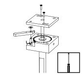
5. Place the black plastic washer over the pin and on top of the ratchet lever and reassemble the lid
