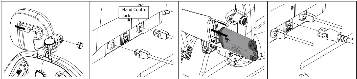
9. Loosen the knob on the articulating headrest mechanism and rotate it forward as shown. Remove the knob on the back of the headrest. Insert the headrest into lock mechanism. Reinsert knob, position headrest as desired, and tighten both knobs.
