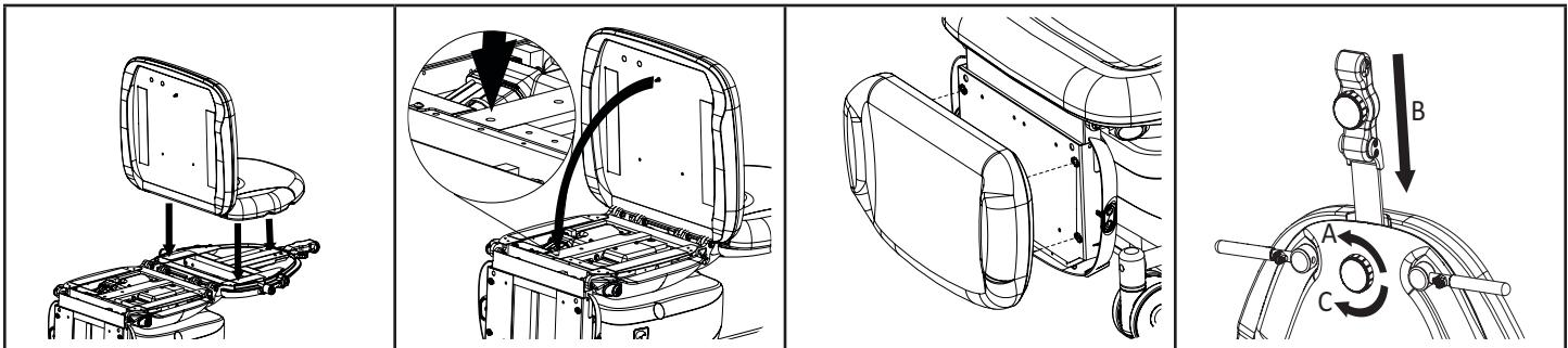
5. With the back and seat sections of the stretcher bed in the flat position, center the back portion of the seat/back cushion on the back section of the stretcher bed while holding up the seat portion of the cushion.
