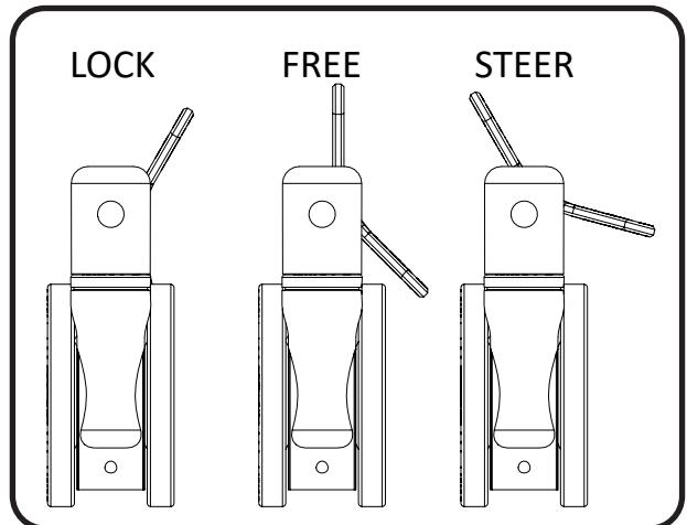
**MODE INDICATOR:** Each locking bar has a mode indicator line on the center of the pedal that points to the adjacent indicator label on the base of the stretcher bed. Note that the (3) Total Lock Casters operate the same whether they are in FREE or STEER Mode.
