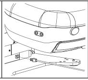
8. (Standard/Non-Lift Base) Plug in the foot control in the foot control jack at the base of the chair. For Swivel Base Chairs see step 9.
