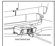
9. (Swivel Base) Plug in the foot control at the base of the chair. Note that the foot control jack is located under the rear cable shroud.
