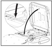
5. Lower the seat portion of the seat/back cushion into place and ensure that the ball stud enters the mating hole in the seat section of the chair.
