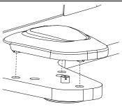
14. Install the (4) leveling glide covers over the feet of the baseplate. Align the snap features over the three holes and press down.
