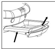
To remove the debris tray, grab the sides of the debris tray and lift up and out.
