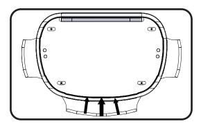
7. Pull the outer tabs of the top and bottom sides of the scuff cover at an angle towards the center and attach to foot cushion velcro to tighten the corner.
