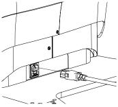
10. Insert the power cord at the base of the chair. Press firmly until it bottoms out. Plug the opposite end of the power cord into an appropriately marked receptacle. See Step 9 image for location of power cord jack in swivel base models.
