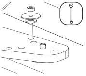
2. Remove (4) shipping bolts with an adjustable wrench or 7/16" end wrench.
