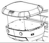
6. Attach the foot cushion by aligning the ball studs to the receptacles and pressing until all 4 snap in place.
