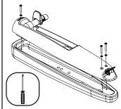
7. Using a screwdriver, attach the arm upholstery to each arm using the provided screws and washers.
