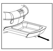
To position the debris tray, grab the handle and pull or push the debris tray to the desired position. When finished, push the debris tray back into the foot section.
