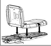
4. With the back and seat sections of the chair in the flat position, center the back portion of the seat/back cushion on the back section of the chair while holding up the seat portion of the cushion.
