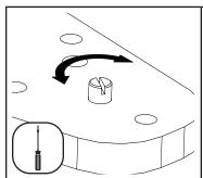
13. Position the chair in the desired location. Level the chair by adjusting the height of the individual leveling glides with a flat head screwdriver.
