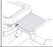
11. Extend the foot section of the chair using the switches on the side of the foot section. Remove the protective film from the chair.
