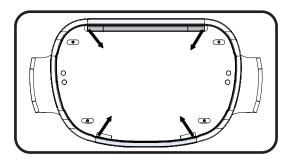
8. Pull at the sides of the scuff cover and fold over the center tabs of the scuff cover and latch them to the velcro on the inside walls.
