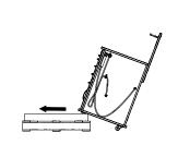
3. Slide the cabinet off the pallet by moving the cabinet on the pallet guides until it is over hanging the back of the pallet. Slide the back of the cabinet off the pallet and pull the pallet out from underneath the cabinet.
