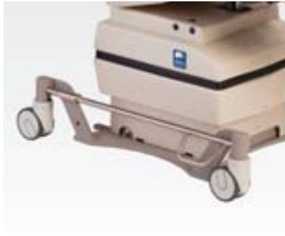
4" (10.2 cm) precision casters with operator selected steering or multidirectional modes make it easy for even one person to steer around corners and the dual braking system locks swivel and rotation of two casters per side simultaneously
